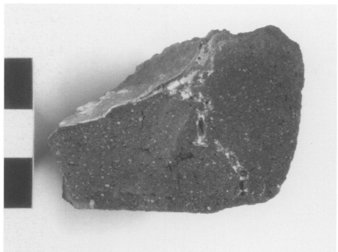
4. Crucible fragment (FZN 92/1227) with glass-filled crack at the heel, running from inside out
